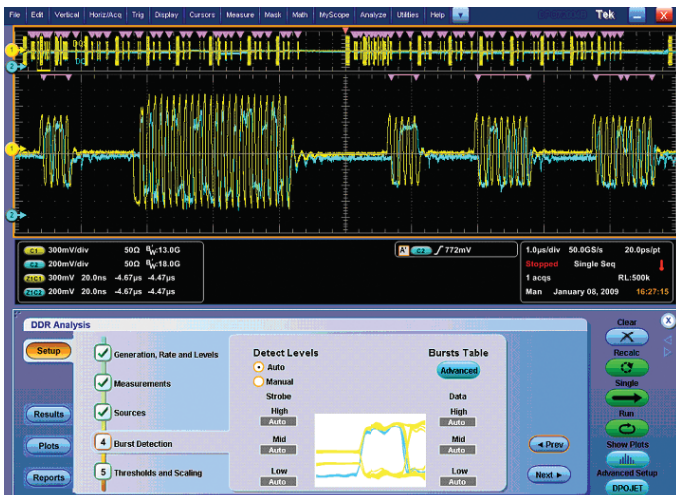
Figure 57. Advanced DDR Analysis tool automates complex memory tasks like separating read/write bursts and performing JEDEC measurements.
