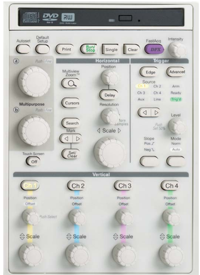
Figure 22. Front-panel control section of an oscilloscope.
