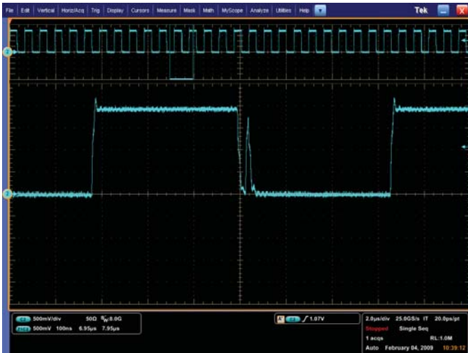
Figure 50. A higher sample rate provides greater signal resolution, ensuring that you'll see intermittent events.
