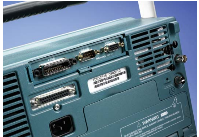
Figure 55. A TDS3000C Series oscilloscope provides a wide array of communications interfaces, such as a standard Centronics port and optional Ethernet/RS-232, GPIB/RS-232, and VGA/RS-232 modules. There is even a USB port (not shown) on the front panel.
